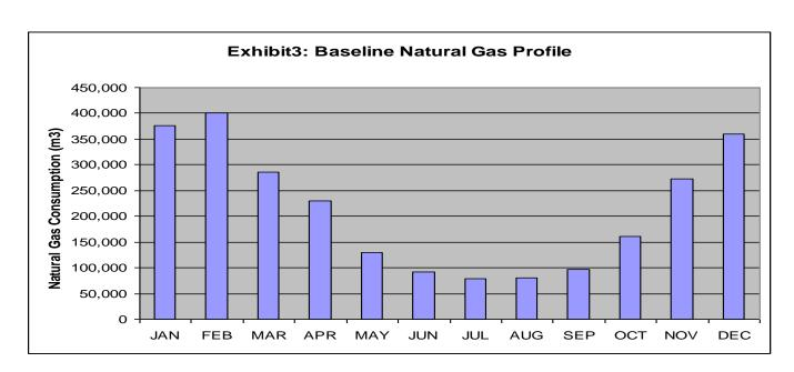
Exhibit 3 shows the monthly natural gas use profile. Approximately one third of the gas is being used for the base load, and there is a predictable winter increase that corresponds well with the heating demand.
