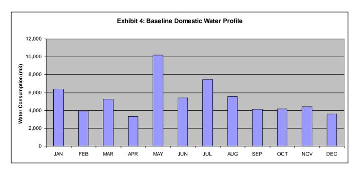
Exhibit 4 shows the monthly water use profile. The majority of the water consumption is base load, but there is an increase in the summer due to cooling loads.
